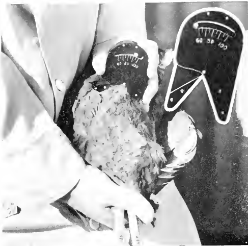
WEST VIRGINIA CHICKEN BREAST METER measures width of bird's breast in degrees. It is taken at the anterior point of the keel in the twelfth week. The meter was developed by the Station in cooperation with the State Department of Agriculture. Will be available in near future.
